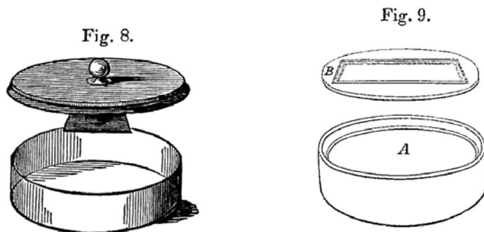
In the centre of the under side of the glass lid, is cemented a small block of wood, to which is attached a piece of sheet Indian rubber, the surface of which is prepared as described for the plate-holder (Fig. 7); the plate is then attached to it in a similar manner. When not in use, a glass cap is placed over the Indian rubber, which effectually prevents any action going on between the vapour from the solution and the Indian rubber.
